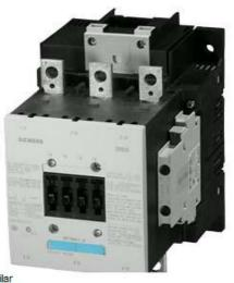
CONTACTOR, 275A/AC-1, AC(40...60HZ)/DC OPERATION UC 23...26V AUX.CONT.2NO+2NC SOLID-STATE COMP., 3-POLE, SIZE S6 BAR CONNECTIONS CONVENT. OPERATING MECHANISM
