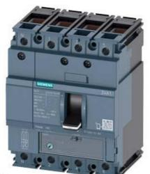
CIRCUIT BREAKER 3VA1 IEC FRAME 160 BREAKING CAPACITY CLASS N ICU=25KA @ 415 V 4-POLE, LINE PROTECTION TM220, ATFM, IN=25A OVERLOAD PROTECTION IR=17,5A ...25A SHORT CIRCUIT PROTECTION II=10 X IN NEUTRAL UNPROTECTED CABLE CONNECTION
