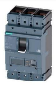
CIRCUIT BREAKER 3VA2 IEC FRAME 630 BREAKING CAPACITY CLASS M ICU=55KA @ 415 V 3-POLE, LINE PROTECTION ETU850, LSI, IN=500A OVERLOAD PROTECTION IR=200A ...500A SHORT CIRCUIT PROTECTION ISD=0,6..10X IN, II=1,5..14X IN NEUTRAL PROTECTION OPTIONAL WITH EXT. CT;UPTO 160% BUSBAR CONNECTION
