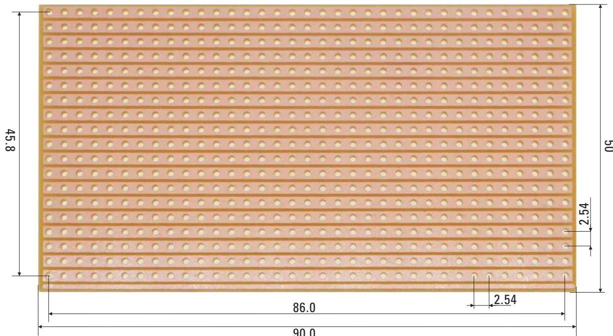
**Material: Synthetic Resin Bonded Paper, FR-1, UL94V-0 (KB3151C)**
