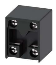
Contact block for position switch 3SE5162 Mounting position on the right in the switch 1 NO/1 NC slow-action contact
