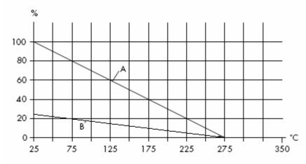
A=mounted on heat-sink B=with no heatsink
