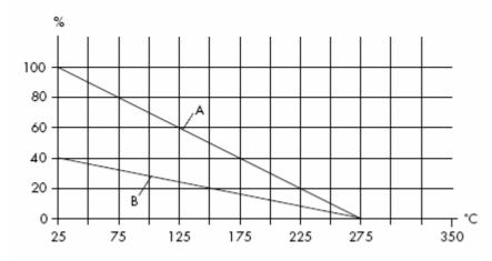
A=mounted on heat-sink B=with no heatsink
