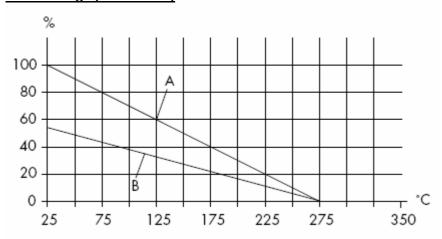
A=mounted on heat-sink B=with no heatsink
