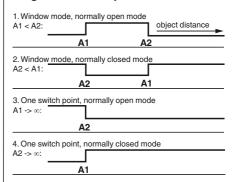
A1 -> ∞, A2 -> ∞: Object presence detection mode Object detected: Switch output closed No object detected: Switch output open
