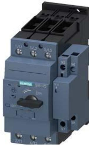
LEISTUNGSSCHALTER BGR. S2, FUER DEN MOTORSCHUTZ, CLASS 10, MIT UEBERLAST-RELAISFUNKTION A-AUSL. 12...17A,N-AUSL. 260A, STANDARDSCHALTVERMOEGEN
