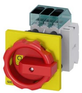
Switch disconnector 3LD3, main switch 3-polig, Iu 63A operational switch at AC-23 A at 400 V 22,0 kW front mounted Base mounting with center-hole 22,5 mm knob-operated mechanism red/yellow 66 x66 mm with auxiliary 1NO+1NC
