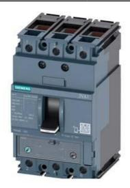
CIRCUIT BREAKER 3VA1 IEC FRAME 160 BREAKING CAPACITY CLASS S ICU=36KA @ 415 V 3-POLE, LINE PROTECTION TM240, ATAM, IN=40A OVERLOAD PROTECTION IR=28A ...40A SHORT CIRCUIT PROTECTION II=5...10 X IN CABLE CONNECTION
