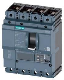
CIRCUIT BREAKER 3VA2 IEC FRAME 100 BREAKING CAPACITY CLASS M ICU=55KA @ 415 V 4POLE, LINE PROTECTION ETU850, LSI, IN=100A OVERLOAD PROTECTION IR=40A ...100A SHORT CIRCUIT PROTECTION ISD=0,6..10X IN, II=1,5..12X IN NEUTRAL PROTECTION ADJUSTABLE (OFF, UPTO 100%) BUSBAR CONNECTION
