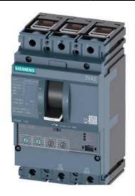
CIRCUIT BREAKER 3VA2 IEC FRAME 100 BREAKING CAPACITY CLASS L ICU=150KA @ 415 V 3POLE, LINE PROTECTION ETU350, LSI, IN=25A OVERLOAD PROTECTION IR=10A ...25A SHORT CIRCUIT PROTECTION ISD=1,5... 10 X IR, II=12 X IN CABLE CONNECTION
