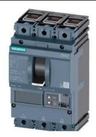
CIRCUIT BREAKER 3VA2 IEC FRAME 100 BREAKING CAPACITY CLASS L ICU=150KA @ 415 V 3POLE, LINE PROTECTION ETU860, LSIG, IN=40A OVERLOAD PROTECTION IR=16A ...40A SHORT CIRCUIT PROTECTION ISD=0,6..10X IN, II=1,5..12X IN NEUTRAL PROTECTION OPTIONAL WITH EXT. CT,UPTO 160% GROUNDFAULT, SWITCHABLE IG=0,2... 1 X IN, TG=0,050,8MS CABLE CONNECTION
