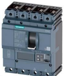
CIRCUIT BREAKER 3VA2 IEC FRAME 100 BREAKING CAPACITY CLASS L ICU=150KA @ 415 V 4POLE, LINE PROTECTION ETU560, LSIG, IN=63A OVERLOAD PROTECTION IR=25A ...63A SHORT CIRCUIT PROTECTION ISD=0,6..10X IN, II=1,5..12X IN NEUTRAL PROTECTION ADJUSTABLE (OFF, UPTO 160%) GROUNDFAULT, SWITCHABLE IG=0,2... 1 X IN, TG=0,050,8MS BUSBAR CONNECTION
