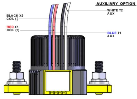
WIRE SPEC: SILICONE, 20AWG, -40C-150C, UL: VW-1
