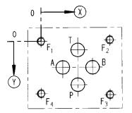
**Mounting hole configuration: NG6** (ISO 4401-03-02-0-94) For subplates see catalog section RE 45053
