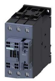
CONTACTOR,AC3:22KW/400V, 1NO+1NC, 220V AC 50/60HZ, 3-POLE, SIZE S2, SPRING-TYPE TERMINAL
