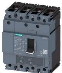
CIRCUIT BREAKER 3VA1 IEC FRAME 160 BREAKING CAPACITY CLASS M ICU=55KA @ 415 V 4-POLE, LINE PROTECTION TM220, ATFM, IN=80A OVERLOAD PROTECTION IR=56A ...80A SHORT CIRCUIT PROTECTION II=10 X IN NEUTRAL PROTECTION 100% BUSBAR CONNECTION
