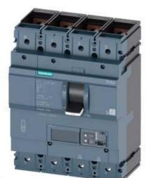
CIRCUIT BREAKER 3VA2 IEC FRAME 630 BREAKING CAPACITY CLASS H ICU=85KA @ 415 V 4-POLE, LINE PROTECTION ETU850, LSI, IN=400A OVERLOAD PROTECTION IR=160A ...400A SHORT CIRCUIT PROTECTION ISD=0,6..10X IN, II=1,5..15X IN NEUTRAL PROTECTION ADJUSTABLE (OFF, UPTO 160%) BUSBAR CONNECTION
