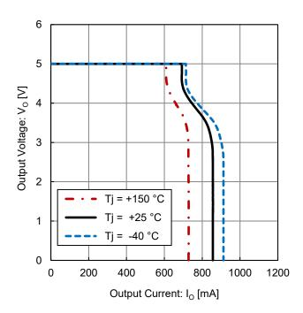
Figure 8. Output Voltage vs Output Current
