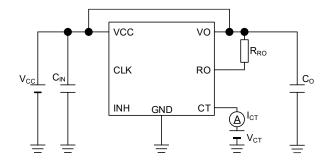
Measurement Setup for Figure 15, 16
