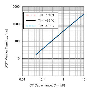
Figure 20. WDT Monitor Time vs CT Capacitance
