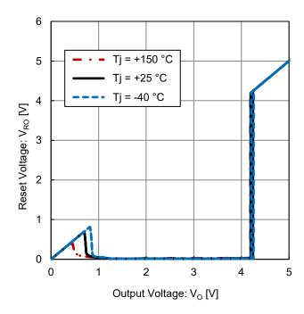
Figure 12. Reset Voltage vs Output Voltage
