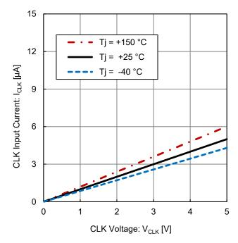
Figure 22. CLK Input Current vs CLK Voltage
