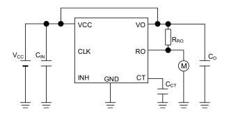
Measurement Setup for Figure 19, 20, 21
