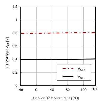
Figure 16. CT Voltage vs Junction Temperature
