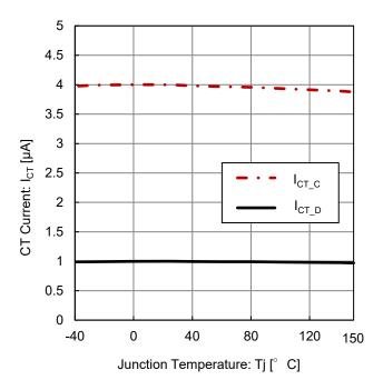
Figure 15. CT Current vs Junction Temperature ( $I_{CT\_C}$ :  $V_{CT}$  = 0.20 V,  $V_{INH}$  = Open  $I_{CT\_D}$ :  $V_{CT}$  = 1.00 V,  $V_{INH}$  = Open)
