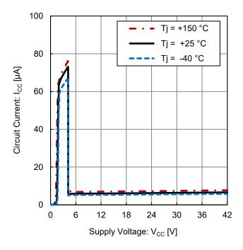
Figure 1. Circuit Current vs Supply Voltage
