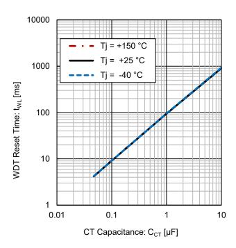
Figure 21. Delay Time vs CT Capacitance
