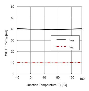
Figure 19. WDT Time vs Junction Temperature
