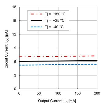
Figure 4. Circuit Current vs Output Current
