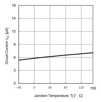
Figure 3. Circuit Current vs Junction Temperature
