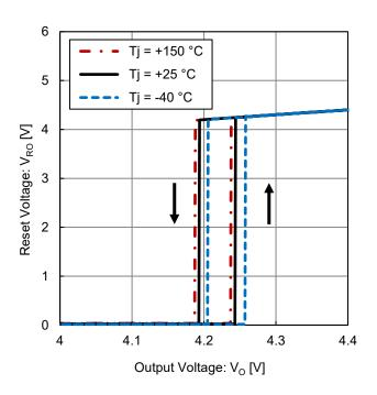
Figure 13. Reset Voltage vs Output Voltage
