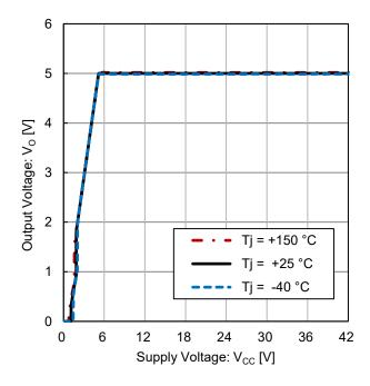
Figure 5. Output Voltage vs Supply Voltage
