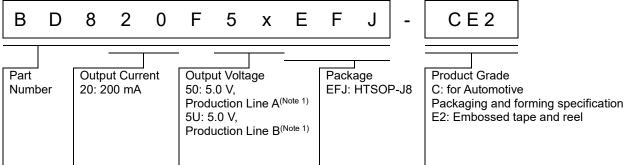
(Note 1) For the purpose of improving production efficiency, Production Line A and B have a multi-line configuration. Electrical Characteristics noted in Datasheet does not differ between Production Line A and B. Production Line B is recommended for new product.
