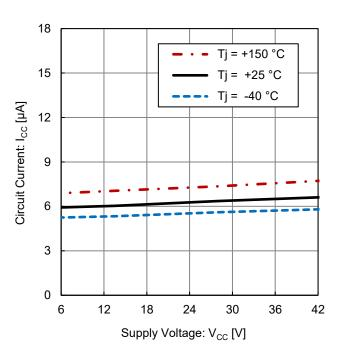
Figure 2. Circuit Current vs Supply Voltage
