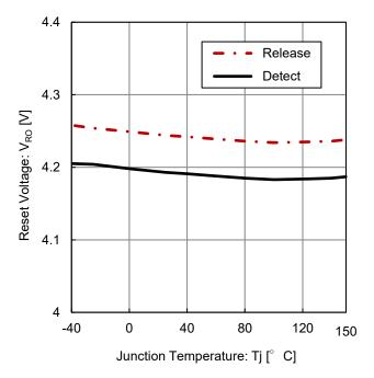
Figure 14. Reset Voltage vs Junction Temperature
