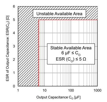
Output Capacitance Co, ESR Available Area (-40 °C ≤ Tj ≤ +150 °C, 5.9 V ≤ V<sub>CC</sub> ≤ 45 V, V<sub>INH</sub> = 5 V, I<sub>O</sub> = 0 mA to 200 mA)
