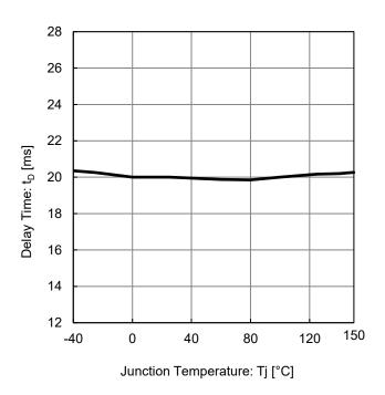
Figure 17. Delay Time vs Junction Temperature
