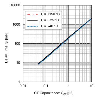
Figure 18. Delay Time vs CT Capacitance
