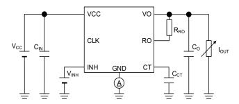
Measurement Setup for Figure 1, 2, 3, 5, 6, 7, 11
