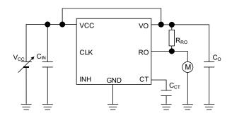
Measurement Setup for Figure 17, 18
