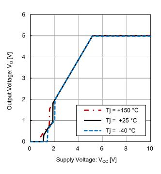
Figure 6. Output Voltage vs Supply Voltage
