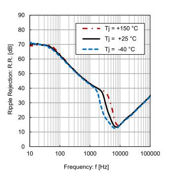
Figure 10. Ripple Rejection vs Frequency (ein = 1 Vrms, I<sub>0</sub> = 100 mA)
