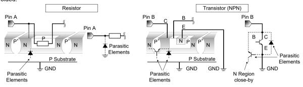
Figure 40. Example of IC Structure
