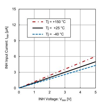
Figure 23. INH Input Current vs INH Voltage
