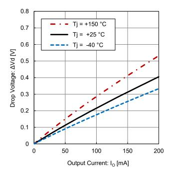
Figure 9. Drop Voltage vs Output Current (Vcc = 4.75 V)
