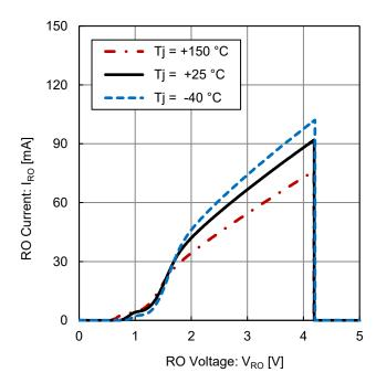
Figure 24. RO Current vs RO Voltage
