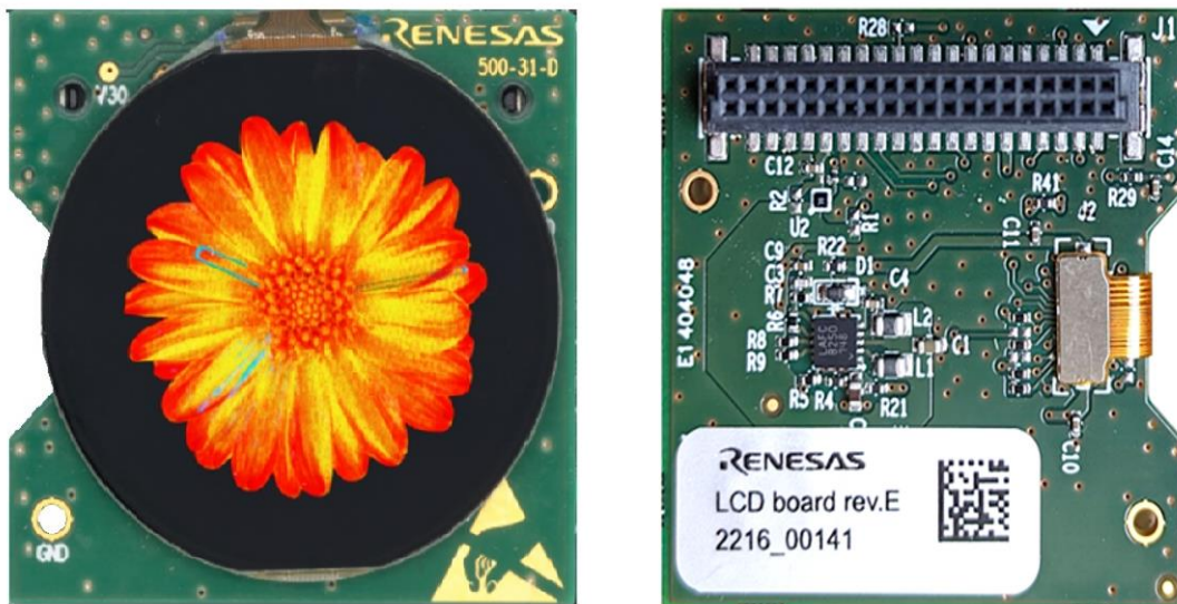
Figure 42: LCD TFT daughterboard top (left) and PCBA bottom side (right)
