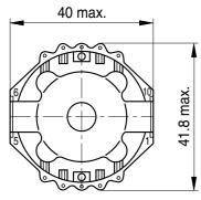
Hole arrangement View in mounting direction
