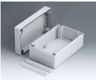
C2112201 ROBUST-BOX 120 BREIT, Ausf. I ABS (UL 94 HB) lichtgrau RAL 7035 200x120x90mm IP 66
