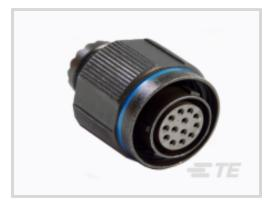
Connector System: Cable-to-Panel Number of Positions: 56 Sealable: Yes Connector & Contact Terminates To: Wire & Cable Contact Current Rating (Max): 13 A
