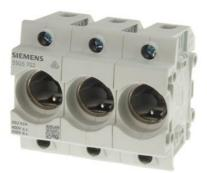
NEOZED, fuse base, D01, 3-pole, 16 A, Un AC: 400 V, Un DC: 250 V without LED signal detector with frame terminal
