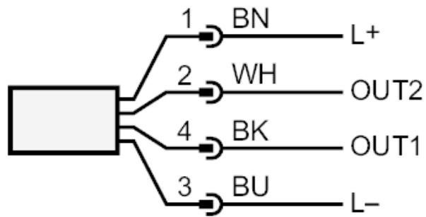
OUT1: switching output IO-Link
