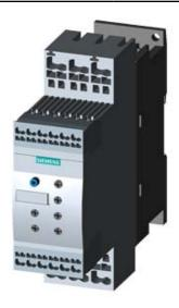
SIRIUS SOFT STARTER, S0, 32A, 18.5KW/500V, 40 DEGR., AC 400-600V, AC/DC 24V, SPRING-LOADED TERMINALS, THERMISTOR MOTOR PROTECTION
