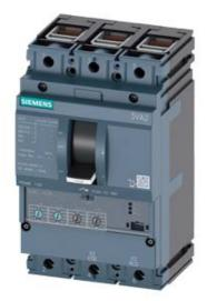
CIRCUIT BREAKER 3VA2 IEC FRAME 100 BREAKING CAPACITY CLASS M ICU=55KA @ 415 V 3POLE, LINE PROTECTION ETU350, LSI, IN=63A OVERLOAD PROTECTION IR=25A ...63A SHORT CIRCUIT PROTECTION ISD=1,5... 10 X IR, II=12 X IN CABLE CONNECTION
