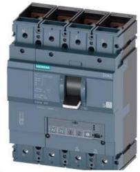
CIRCUIT BREAKER 3VA2 IEC FRAME 400 BREAKING CAPACITY CLASS M ICU=55KA @ 415 V 4-POLE, LINE PROTECTION ETU350, LSI, IN=250A OVERLOAD PROTECTION IR=100A ...250A SHORT CIRCUIT PROTECTION ISD=1,5... 10 X IR, II=12 X IN NEUTRAL PROTECTION ADJUSTABLE(OFF,50%,100%) BUSBAR CONNECTION
