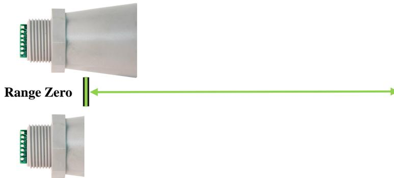
The range is measured from the front of the transducer.
