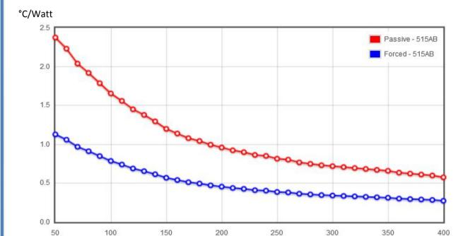
Thermal Resistance is calculated based on a distributed heat load and vertically mounted fins anodised heatsink with a 60°C temperature.
