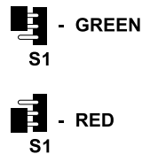
Figure 2.11 i/8 D Location of S1 and Selectable Jumper Positions
