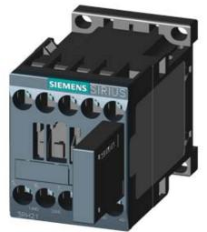
COUPLING CONTACTOR RELAY, 2NO+2NC, DC 24V, 0.85..1.85\*US, W/ PLUGGED-ON VARISTOR, SIZE S00, SCREW TERMINAL
