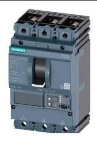
CIRCUIT BREAKER 3VA2 IEC FRAME 100 BREAKING CAPACITY CLASS L ICU=150KA @ 415 V 3POLE, LINE PROTECTION ETU550, LSI, IN=63A OVERLOAD PROTECTION IR=25A ...63A SHORT CIRCUIT PROTECTION ISD=0,6..10X IN, II=1,5..12X IN NEUTRAL PROTECTION OPTIONAL WITH EXT. CT,UPTO 160% BUSBAR CONNECTION
