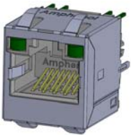
P/N RJE45-188-1XX1 SHOWN SINGLE PORT, 8 POSITION, WITH SHIELD AND LEDs CAT6
