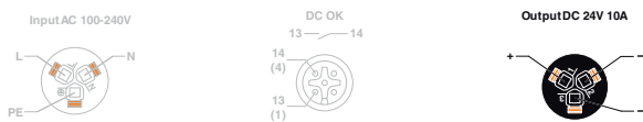
Figure 19 Device-side position and contact assignment of the IPD panel feed-through connector (black) Output DC
