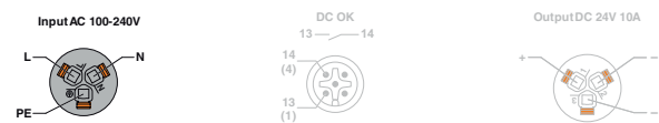
Figure 16 Device-side position and contact assignment of the IPD panel feed-through connector (gray) Input AC
