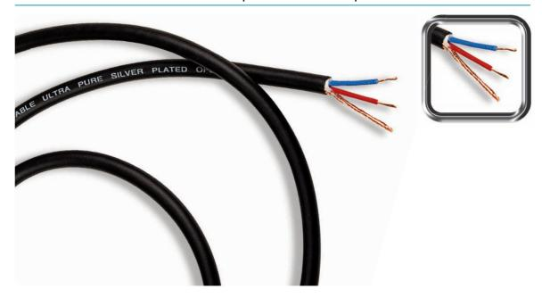
Van Damme Super Flexible 1 pair is a 3.60mm balanced analogue audio cable with a lapped copper spiral screen. This cable is ideal for use with miniature connectors such as the Switchcraft Tini-Qg range and other small connectors typically found on Lavalier microphones. Its helical spiral shield can withstand multiple flexing operations making it preferable to foil screened 1 pair for certain dynamic applications
