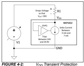
FIGURE 4-2: V<sub>DD</sub> Shunt.
