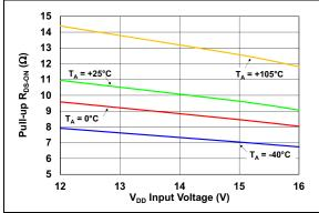
**FIGURE 2-16:** Output High-Side Transistor *R*<sub>DS-ON</sub> vs. *V*<sub>DD</sub> Input Voltage.
