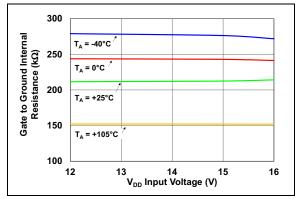
**FIGURE 2-20:** Gate to Ground Internal Resistance vs. V<sub>DD</sub> Input Voltage.
