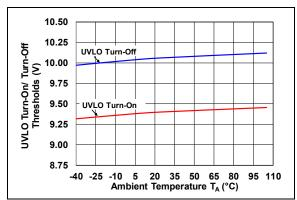
**FIGURE 2-4:** UVLO Turn-Off and Turn-On Thresholds vs. Temperature.
