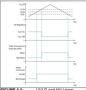
**FIGURE 4-1:** UVLO and HV Linear Regulator Turn-Off Thresholds.
