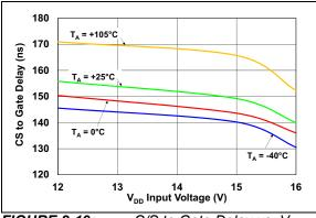
FIGURE 2-19: C/S to Gate Delay vs. V<sub>DD</sub> Input Voltage.
