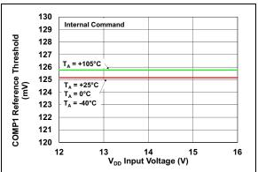
**FIGURE 2-12:** COMP1 Reference During Internal Command vs. V<sub>DD</sub> Input Voltage.
