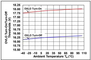
FIGURE 2-5: OVLO Turn-On and Turn-Off Thresholds vs. Temperature.
