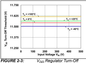
Threshold vs. V<sub>IN</sub> Voltage.
