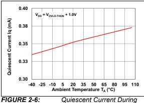
**FIGURE 2-6:** Quiescent Current During OVLO vs. Temperature.
