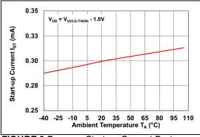
**FIGURE 2-7:** Start-up Current During UVLO vs. Temperature.
