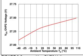
**FIGURE 2-8:** V<sub>DD</sub> OVP2 Voltage vs. Temperature.
