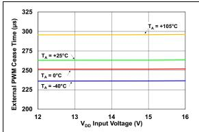
**FIGURE 2-14:** External PWM Cease Time vs. V<sub>DD</sub> Input Voltage.
