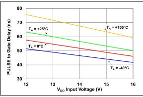
**FIGURE 2-18:** PULSE to Gate Delay vs. V<sub>DD</sub> Input Voltage.
