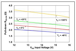
**FIGURE 2-17:** Output Low-Side Transistor R<sub>DS-ON</sub> vs. V<sub>DD</sub> Input Voltage.
