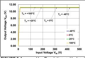
**FIGURE 2-1:** V<sub>DD</sub> Regulation vs. V<sub>IN</sub> Input Voltage.
