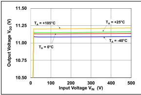
**FIGURE 2-2:** V<sub>DD</sub> Regulation vs. V<sub>IN</sub> Input Voltage (Zoomed Image).
