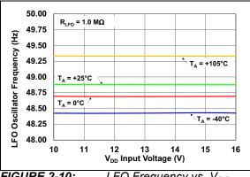
**FIGURE 2-10:** LFO Frequency vs. V<sub>DD</sub> Input Voltage.
