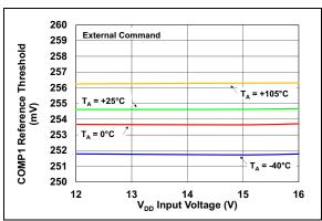
**FIGURE 2-11:** COMP1 Reference During External Command vs. V<sub>DD</sub> Input Voltage.
