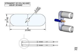
W14020G is specially designed for stripping high-temperature wire insulations made of thermostable materials such as Teflon\*, Kapton\*, silicone rubber, etc, of 20 AWG (0.81 mm / 0.0319 in).
