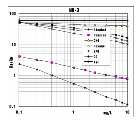
According to the figure, we can see that the minimum concentration we can test is 0.1mg/L and the maximum is 10mg/L. However, we can't provide a formula because the relation between ratio and concentration is nonlinear.
