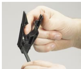
Insert cable, rotate and pull of scrap
