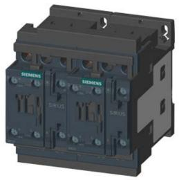
REV. COMB., AC3, 7.5KW/ 400V AC110V 50HZ/120V 60HZ 3-POLE, SZ S0 SCREW TERMINAL ELECTR. AND MECH. INTERLOCK 2NO INTEGR.
