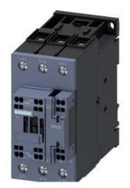
CONTACTOR,AC3:30KW/400V, 1NO+1NC, 20-33V AC/DC, 3-POLE, SIZE S2, SPRING-TYPE TERMINAL
