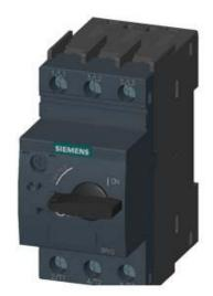
CIRCUIT-BREAKER SZ S0, FOR MOTOR PROTECTION, CLASS 10, A-RELEASE 14...20A, N-RELEASE 260A, SCREW CONNECTION, STANDARD SW. CAPACITY,
