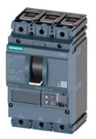
CIRCUIT BREAKER 3VA2 IEC FRAME 100 BREAKING CAPACITY CLASS H ICU=85KA @ 415 V 3POLE, LINE PROTECTION ETU560, LSIG, IN=25A OVERLOAD PROTECTION IR=10A ...25A SHORT CIRCUIT PROTECTION ISD=0,6..10X IN, II=1,5..12X IN NEUTRAL PROTECTION OPTIONAL WITH EXT. CT,UPTO 160% GROUNDFAULT, SWITCHABLE IG=0,2... 1 X IN, TG=0,050,8MS CABLE CONNECTION
