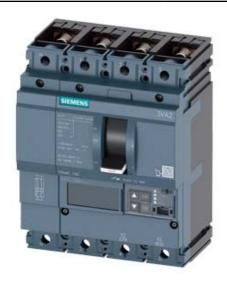
CIRCUIT BREAKER 3VA2 IEC FRAME 160 BREAKING CAPACITY CLASS C ICU=110KA @ 415 V 4POLE, LINE PROTECTION ETU560, LSIG, IN=100A OVERLOAD PROTECTION IR=40A ...100A SHORT CIRCUIT PROTECTION ISD=0,6..10X IN, II=1,5..12X IN NEUTRAL PROTECTION ADJUSTABLE (OFF, UPTO 160%) GROUNDFAULT, SWITCHABLE IG=0,2... 1 X IN, TG=0,050,8MS BUSBAR CONNECTION
