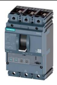
CIRCUIT BREAKER 3VA2 IEC FRAME 250 BREAKING CAPACITY CLASS M ICU=55KA @ 415 V 3POLE, LINE PROTECTION ETU330, LIG, IN=160A OVERLOAD PROTECTION IR=64A ...160A SHORT CIRCUIT PROTECTION II=1,5...12 X IN GROUNDFAULTPROTECTION IG=0,2... 1 X IN, TG=0,1/0,3MS BUSBAR CONNECTION
