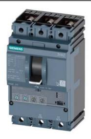
CIRCUIT BREAKER 3VA2 IEC FRAME 250 BREAKING CAPACITY CLASS C ICU=110KA @ 415 V 3POLE, LINE PROTECTION ETU350, LSI, IN=250A OVERLOAD PROTECTION IR=100A ...250A SHORT CIRCUIT PROTECTION ISD=1,5... 10 X IR, II=10 X IN BUSBAR CONNECTION
