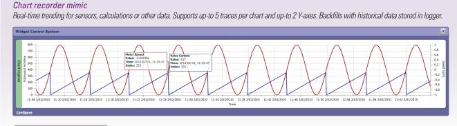
USB port equipped models only. dEX operates on all DT80 range Series 2 & Series 3 models (DT80, DT81, DT82E, DT85, DT80G, DT85G). The latest firmware which includes dEX is available for download from the dataTaker website. DT80 range Series 1 models do not support dEX
