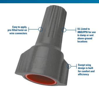
Designed specifically for above ground, interior/exterior connections exposed to damp/wet and corrosive environments. WeatherProof® connectors are pre-filled with a non-hardening, silicone-based gel that protects against moisture and corrosion.
