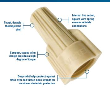
The No.1 twist-on wire connector. The Twister® easily handles the most common wiring tasks. A patented, expanding square-wire spring always ensures a quick, safe connection.
