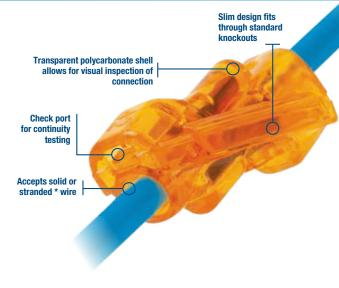
SpliceLine® in-line wire connectors provide a crimp-free, solderless butt splice. Accepts a broad range of wire sizes, allowing one connector to do the job of multiple through-crimps. Its end-to-end connection is also a great solution for pre-fab operations
